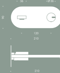
7305/3/1 Miscelatore per lavabo a muro su piastra, L 210 Wall mounted single lever mixer for basin, L 210
