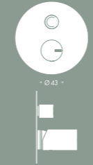
7300 Miscelatore incasso c/pulsante 2 OUT Built-in single lever mixer with diverter pulse 2 OUT
